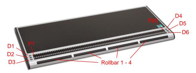
VarioPro does not require its own on/off switch and is powered from the PC or from the mains adapter. As soon as VarioPro receives power it switches itself on and emits a corresponding tone.
