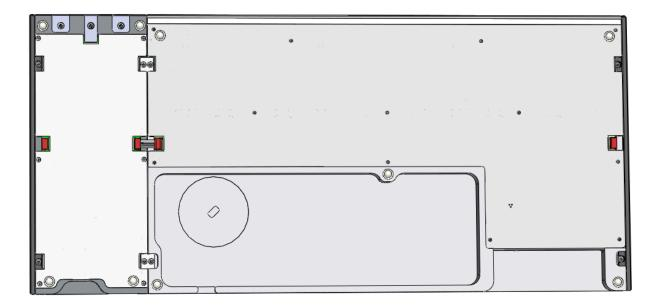
Remove corresponding side-covers from VarioPro and TASO and instead of this make the mechanical connection with the "Connector" (accessory TASO) by using the same screws. Make the electrical connection by plug-in the delivered "Module-bridge" (accessory TASO).
