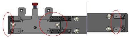
Change the side of the pin-connector by temporary loosening the cross-recess screw and moving board.
