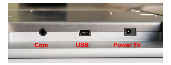
The communication channels/ports are located in the recess at the back of the device on the right, approximately 2cm deep. On the far left is the round socket for the COM port; in the middle the square socket for the USB port (mini-USB port) and on the far right the mains adapter socket (5 volt).
