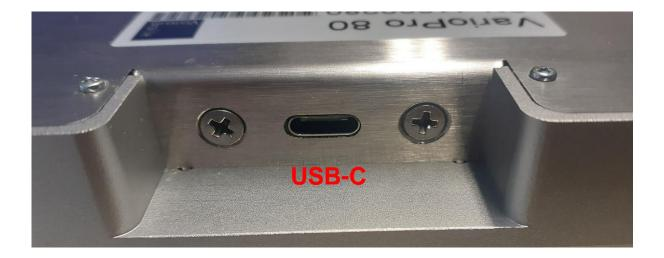
The USB-C connection socket (for connecting to a computer, laptop or notebook) is about 2 cm embedded in a recess on the left rear of the housing.
