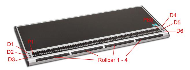
VarioPro2 does not require its own on/off switch and is powered from the PC. As soon as VarioPro2 receives power it switches itself on and emits a corresponding tone.
