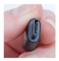
On the left side of Vario 340 you can find the USB port, which is USB type C. Special about the USB Type C port is, that it doesn't matter which direction the USB plug is facing. No more finding the right position of the plug.
