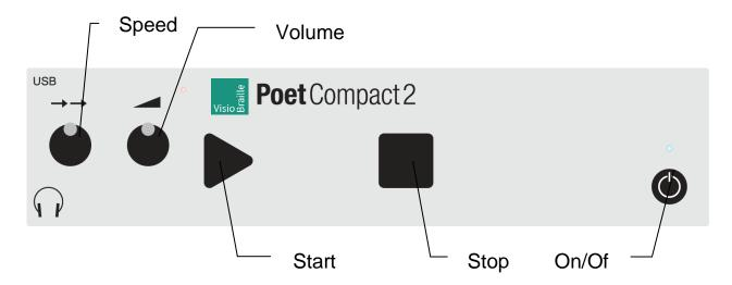
The buttons and loud speakers are located on the front side of the reading machine. The cover of the scanner is located on the top, the mains connector jack and the transportation lock are located on the rear.
